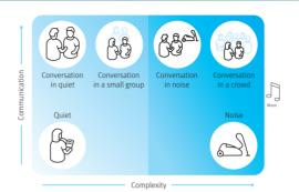
Integra OS, the engine that operates the hearing aids, classifies sounds into a range of seven key listening environments – from very quiet to complex situations, with and without speech. It automatically optimises the listening experience, blending environments into a unique combination appropriate for each situation.
